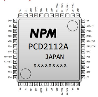
Note: No. 1 pin is located at the bottom left with the type name making "1".
