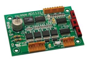
Nippon Pulse's AD1131 is a constant voltage driver board designed for 2-phase unipolar stepper motors.
