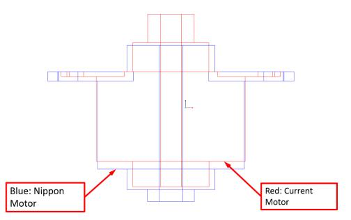
Shape modifications from our standard motor (blue line drawing) to fit the shape of application's current motor (red line drawing).
