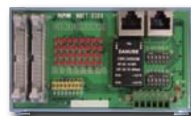
MNET-304 Local Output Board (Isolated 32 outputs)
