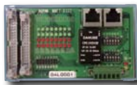
MNET-322 Local Input/Output Board (Isolated 16 inputs/outputs)
