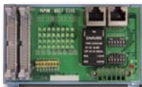
MNET-340 Local Input Board (Isolated 32 inputs)
