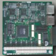
NPMCMMNET-I/O104 PC/104 Bus Center Board (G9001A x 2)
