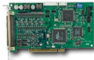
PPCI-7443 Quadaxial Motion Control Board with PCI Bus
